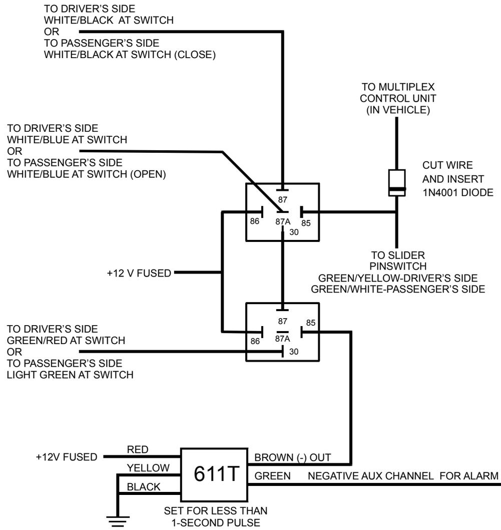
Set 611T for less than one second pulse, set dip switches as follows:
