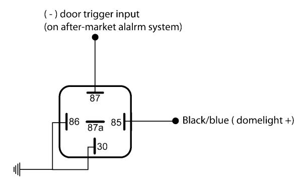
On some Ford's, there is a problem with false alarms when an after-market alarm is installed and connected to the Domelight wire for door supervision. This is caused by diagnostic pulses send down the wire by the vehicle's GEM module. The solution is to add a relay. This will isolate these pulses yet still allow the dome-light to be used for door supervision.
