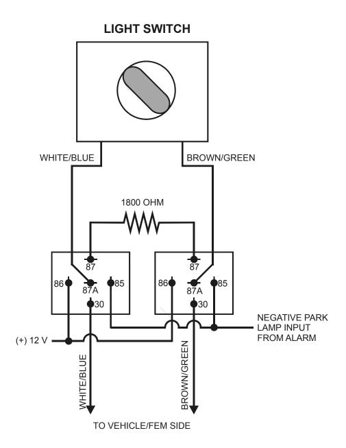
**IMPORTANT!** This wiring information is being provided free of charge on an "as is" basis, without any representation or warranty. It is the dealer's responsibility to verify any circuit before interfacing with it using a digital multi-meter. Directed Electronics Inc. assumes no responsibility with regards to the accuracy or currency of this information. Proper installation in every case remains the responsibility of the installer.
