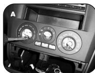
Unsnap top section of panel below climate controls. It is not necessary to fully remove panel.
