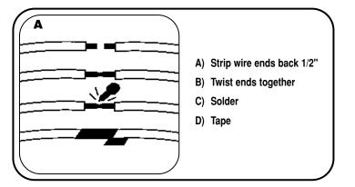
1 Locate the factory wiring harness in the dash. Metra recommends using the proper mating adapter and making connections as shown. (Isolate and individually tape off the ends of any unused wires to prevent electrical short circuit.)
