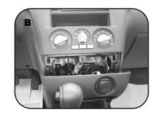
Remove (4) phillips screws to remove radio. **5**
