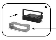
Slide the DIN cage into the **Radio Housing** and secure by bending the metal locking tabs down.
