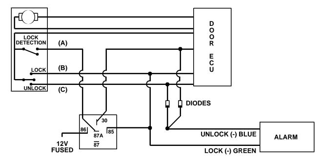
**NOTE:** To unlock all the doors with a single pulse this interface must be wired in the passenger door. To have progressive unlocking, or if using a unit with double pulse unlock, this interface may be wired in the driver door. The Toyota Avalon, however, will not work with the double pulse. The charts below show the corresponding wires.
