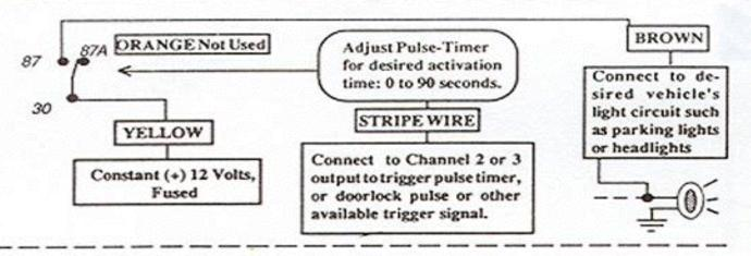
If you need to disconnect a circuit for a certain amount of time, so that the alarm does not activate, you can use the pulse-timer's normally closed circuit, pulse the stripe wire to disconnect the circuit for up to 90 seconds.
