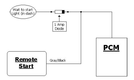
When tying in to the glow plug wire, install a 1 amp diode on the factory wire to prevent the wait to start light from backfeeding ground to the remote start.
