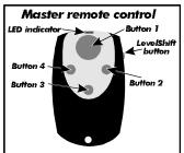
*To transmit either channel 1, 2, 3 or 4:* Just press either button 1, 2, 3 or 4. While you transmit, the LED indicator *on the remote control* will flash once every second: this indicates **level 1**.
