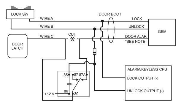
**NOTE:** When testing the Door Ajar wire, it will rest at ground when the door is closed and pulse to (+) 12 volt when the door opens then return to ground. This diagram will also activate the dome light upon unlock.
