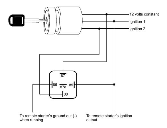
If your vehicle has a second ignition wire that must be powered during remote start, using a relay will keep the 2 ignition wires isolated from each other.
