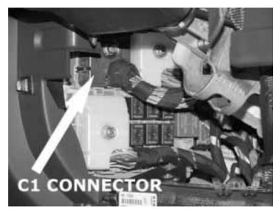
This 1-wire doorlock system requires resistors. The values indicated are the exact values from Jeep. You can go higher or lower by about 5-10% and it should still work fine. The Fuseblock is located directly below the driver's side of the dash. The lower panel is clipped in place (no screws to remove). Relays are used to provide a good ground since the transistorized doorlock outputs from some after-market systems are not sufficient.
