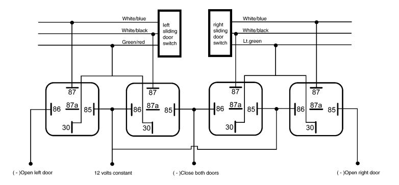
The sliding door switches are in the dashboard to the left of the steering column. The doors must be unlocked before they can be opened. If only one door is needed, you can eliminate the 2 relays under the switch you don't need.
