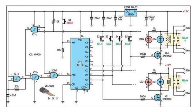
This simple circuit performs exactly the same job. It can be configured with any number of outputs between two and nine, simply by adding pushbutton switches and relay driver circuits to the currently unused outputs of IC2 (O5-O9).
